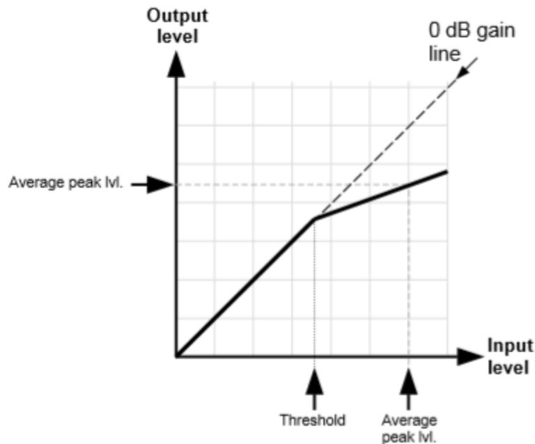
In this operation the desired reduction of the dynamics is performed, but the total loudness is reduced as well. The average peak level is considerably reduced. Usually, the loudness reduction is not a desired effect, and unexpected from sound compression.
