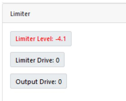
The **Limiter** settings are crucial for an optimised audio output level. If the audio output from the compressor does not reach the *Limiter Level*, the output peaks will not be at the desired and set *Peak Level*. This is because the *Limiter Level*, will be transformed to the user defined *Peak Level* by an automatic function in the *Alignment* procedure.
