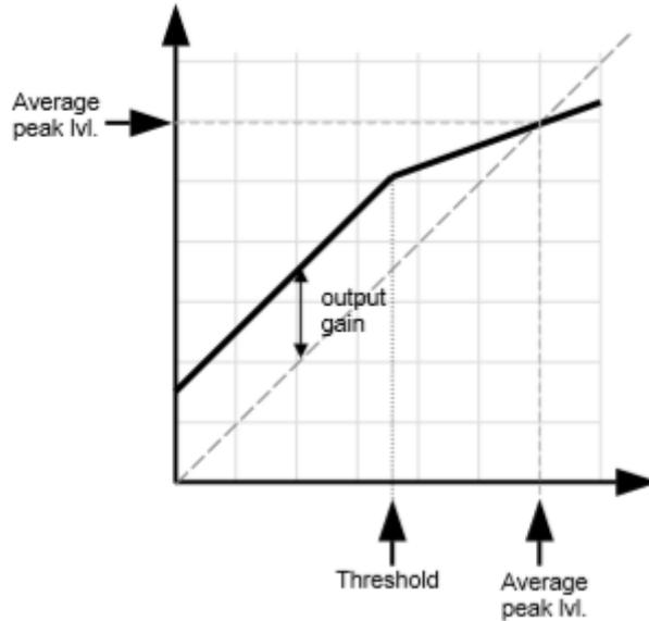
Furthermore, it is likely a constant average peak level is wanting to be maintained when trimming and adjusting the parameter settings. Also, when checking the compression effect by switching it on and off. To accomplish this, repeated output gain or fader corrections are needed.
