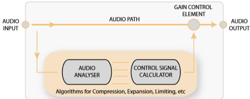
The Compressor action is adapted to human hearing instead of being a purely technical gain servo system. The parameters preserve the original impression of dynamics and life of the sound: Beat music still has a driving beat at the compressor output.
