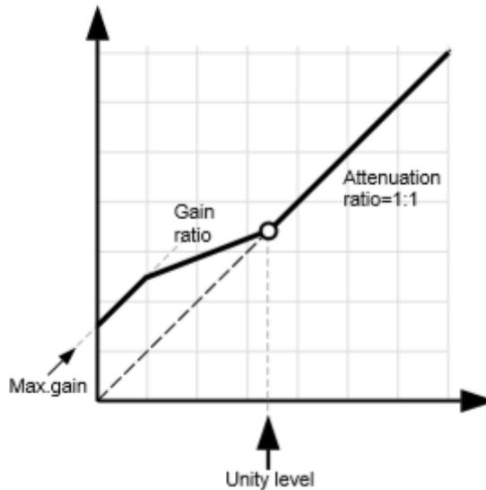
CADENZA has separate ratio settings below and above the *Unity Level* pivot. The *Gain Ratio* setting controls the gain below the pivot, while the *Attenuation Ratio* setting controls the attenuation above the pivot. This feature, along with lowering the *Unity Level*, are the absolute conditions for creating the unique combination of low-level compression and linear dynamics at loud sound passages.
